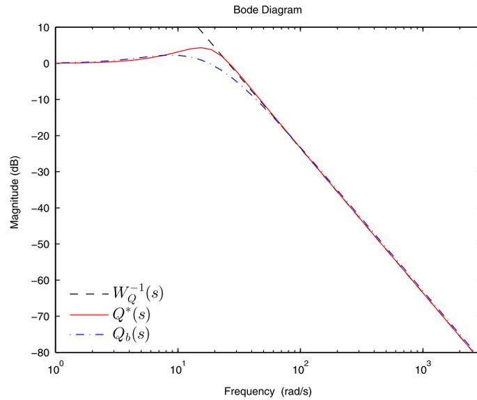
Figure 3. Frequency magnitude responses of  $W_Q^{-1}(s)$ ,  $Q^*(s)$  and  $Q_b(s)$ .
