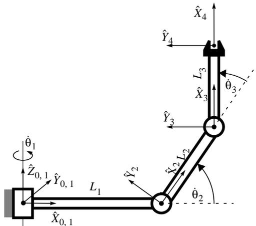
robot joint variables. This underdetermined system of equations must have interdependencies among the elements of  $\dot{X}$ .
