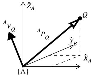
The position of a point Q in {A} is represented by the linear position vector,  ${}^A P_Q$ :
