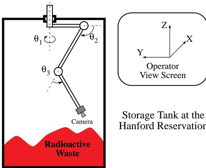
the robot motions in frame {4} which is fixed relative to the camera view. A computer system interprets the operator's commands and computes the necessary joint velocities to achieve the commanded cartesian motion using the relation
