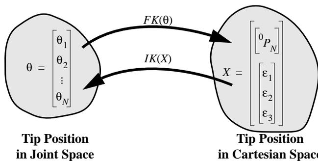
The robot kinematics equations relate these two descriptions of the robot tip position. Specifically, the forward kinematics,  $X = FK(\theta)$ , allows us to determine the cartesian position given the joint positions, while the inverse kinematics,  $\theta = IK(X)$  allows us to determine the necessary joint positions to achieve a desired cartesian position.
