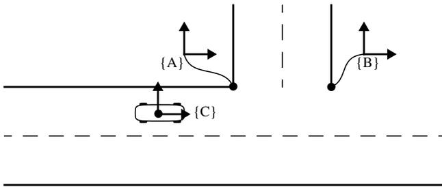
As long as {A} and {B} are fixed relative to each other and have the same orientation, the velocity is unchanged. For this reason, linear velocity vectors are called free vectors.
