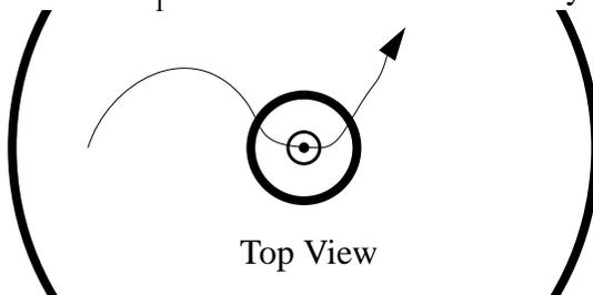
Jacobian will be singular when the robot tip frame {4} intersects the axis of  $\theta_1$  and that the robot will be unable to move along the  ${}^4z$  axis since the third row of the Jacobian becomes all zeros. But what happens when the robot is *approaches* the singularity condition?
