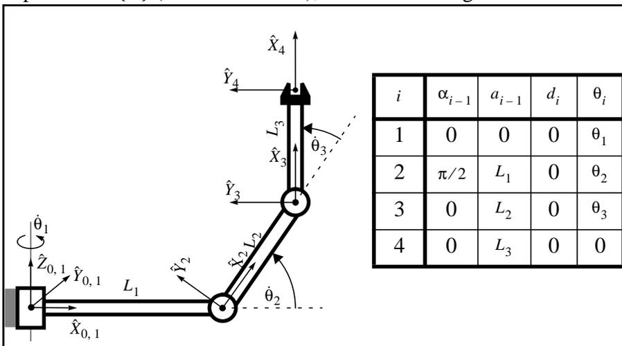
Using techniques derived in earlier parts of this class, we can specify the homogeneous transform matrix  ${}_{i+1}^i T$  for each adjacent link pair:
